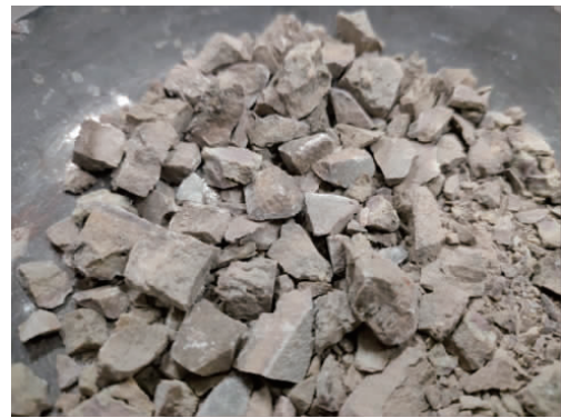
图 8 优选条件下制备的铝酸钙精炼渣 Fig. 8 Calcium aluminate refining slag prepared under optimal conditions
